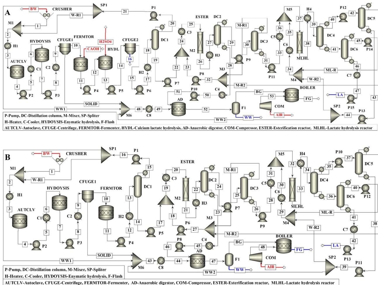
Fig. 1 Flowsheet without process integration for microbial production of lactic acid (LA) from bread waste (BW) under (A) acid-neutral condition (Scenario I) and (B) low pH condition (Scenario II) with a feeding rate of 100 MT BW per day.
