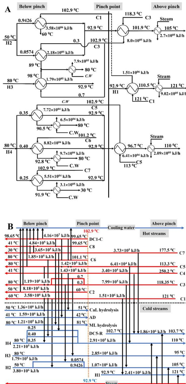
Fig. 3 (A) Heat exchanger network (HEN) and (B) grid diagram for fermentative production of lactic acid (LA) from bread waste (BW) using acid-neutral microorganisms (Scenario I).
