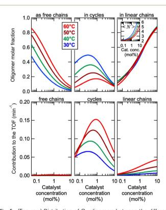
Fig. 5 (Top row) Distribution of  $O_a$  oligomers between the different co-existing species in the  $O_a/O_{bi}$  systems (i=1 or 2), depending on temperature and concentration, computed from the model. The inset in the right graph is the average degree of poly(oligomerization) by number of the linear chains vs. catalyst concentration. (Bottom row) Contribution of the different co-existing species to the catalytic turnover frequency, in the complete  $O_a/O_{b1}$  system.
