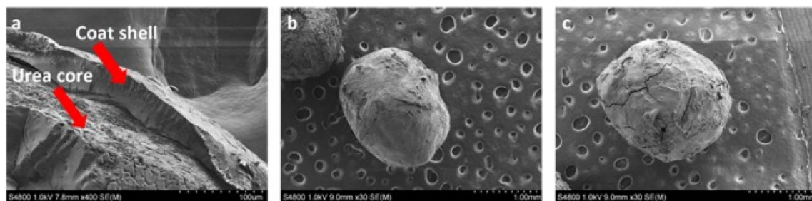
Fig. 13 SEM images of PLA-lignin coated urea pellets showing (a) the coating layer over urea core and the coated pellet (b) before and (c) after urea release to surrounding water. This figure has been adapted/reproduced from ref. 144 with permission from Elsevier B.V., copyright 2017.
