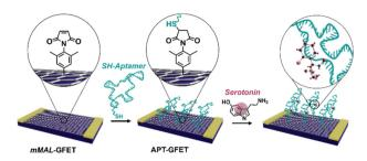
Fig. 1 Schematic of the aptamer conjugation on functionalized GFETs (mMAL-GFETs) and subsequent serotonin recognition.
