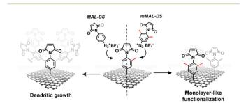
Fig. 2 Schematic of the functionalisation using mMAI -DS (right) and MAL-DS (left) leading to monolayer-like and dendritic-like functionalisation, respectively.
