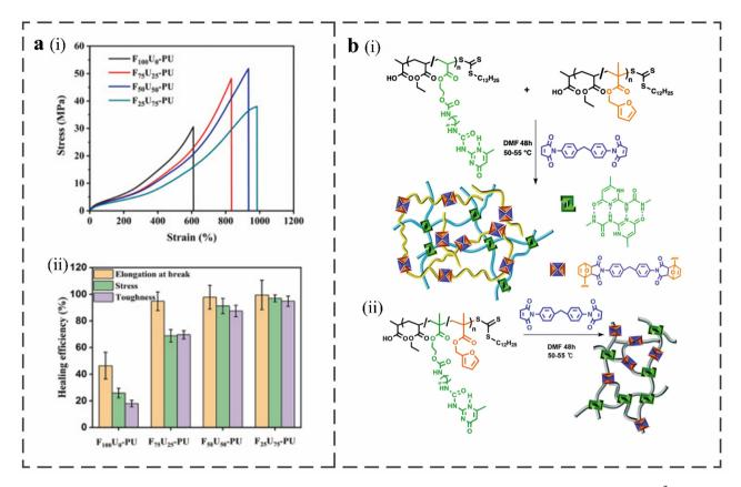
Fig. 4 (a), (i) Typical stress–strain curves of FaUb-PU. (ii) Healing efficiency of breaking strain, stress, and toughness of FaUb-PU. (i) Crosslinkers and polymers used in the preparation of RAFT based IPN (i) and SN (ii) materials. Slashes indicate random incorporation of monomers.<sup>9</sup>
