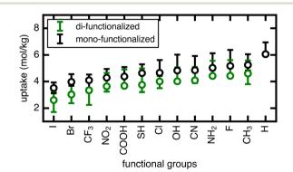
Fig. 5 Range of methane uptake (in mol kg<sup>-1</sup>) at 298 K and 65 bar in UiO-66 with mono- and di-functionalized BDC linkers. 13 different functional groups were studied. Circles represent the uptakes of methane in structures with unrotated linkers and whiskers indicate maximum and minimum values. The functional groups are ordered on the x-axis by increasing uptake of corresponding mono-functionalized structures with unrotated linkers from left to right.
