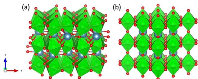
**Fig. 2** Orthorhombic (a) and cubic (b) structure of CaZrO<sub>3</sub>. Ca, Zr and O atoms are represented by blue, green and red spheres, respectively. ZrO<sub>6</sub> octahedra are indicated in green.
