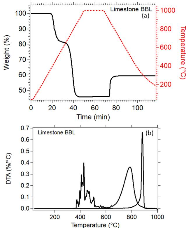
Fig. 7 (a) TGA of Lim BBL in N<sub>2</sub> environment up to 1000 °C (b) DTA of Lim BBL in N<sub>2</sub> environment up to 1000 °C.
