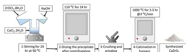
Fig. 1 Illustration of the CaZrO<sub>3</sub> nanoparticle synthesis method.
