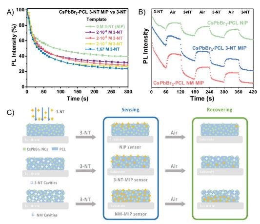
Fig. 5 (A) Real-time response of the CsPbBr<sub>3</sub>-PCL nanocomposite imprinted with different concentrations of 3-NT upon exposure to 3-NT vapours. (B) Real-time response of the CsPbBr<sub>x</sub>-PCL NIP and CsPbBr<sub>x</sub>-PCL 3-NT and NM MIP sensors under repeated exposure cycles to 3-NT vapours (grey areas) and air (white areas). (C) Schematic representation of the NIP/MIP sensing process.
