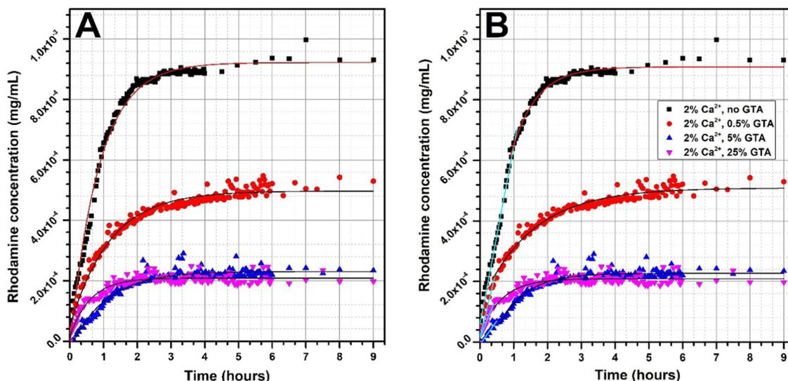
Fig. 7 Rhodamine 640 release profile from GAMS cross-linked with different methods with model fitted curves: (A) exponential fit for all the data, (B) linear fit for the initial period of releasing and exponential fit for the following data.
