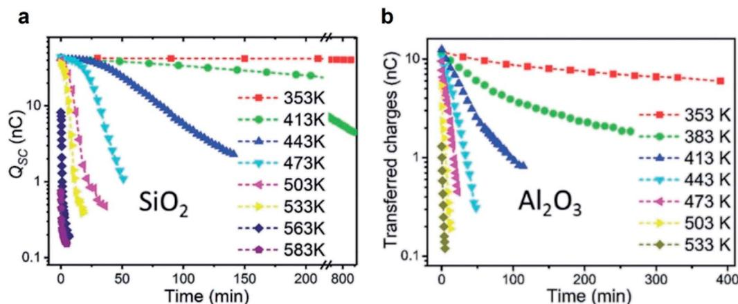
Fig. 8 Charge dissipation by thermionic emission. Amounts of static charge on (a)  $\text{SiO}_2$  and (b)  $\text{Al}_2\text{O}_3$  surfaces as a function of time under different temperatures. Reproduced with permission (copyright 2018, Wiley-VCH).<sup>122</sup>
