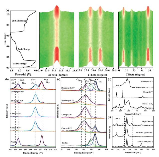
Fig. 3 (a) In situ XRD patterns of Sb<sub>2</sub>S<sub>3</sub> electrodes in different charge/discharge states. (b and c) Ex situ XPS spectra of Sb 3d and S 2p of Sb<sub>2</sub>S<sub>3</sub> electrodes in different charge/discharge states. (d) Ex situ Raman spectra of Sb<sub>2</sub>S<sub>3</sub> electrodes in different charge/discharge states. (e) Raman spectra of the electrolyte after fully charged sate, pure electrolyte, and electrolyte with SbCl<sub>5</sub>.
