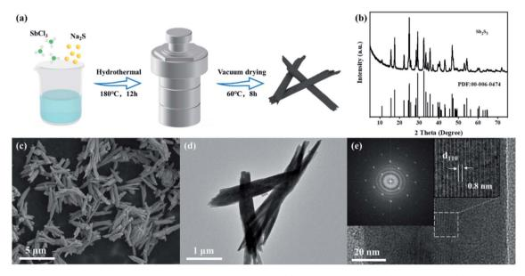
Fig. 1 (a) Schematic diagram of the preparation process of  $Sb_2S_3$  nanorods. (b) XRD pattern; (c) SEM; (d) TEM image; (e) HR-TEM image and the selected-area electron diffraction pattern of  $Sb_2S_3$ .
