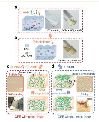
Fig. 1 Preparation schematic of the gel polymer electrolyte (GPE). (a) The complexation of the AAM monomer with  $AlCl_3$  in DCM solvent. (b) Introducing abundant ionic liquid (IL). (c) The GPE polymerized with an MBAA cross-linker delivering a bubble-free and self-support membrane. (d) Typical fabrication showing a sticky GPE with bubbles.
