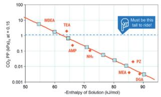
Fig. 4 Solvent ranges of viability. Image adapted with data from Mathias, Int. J. Greenh. Gas Control, 2013, 19, 262–270.<sup>53</sup>
