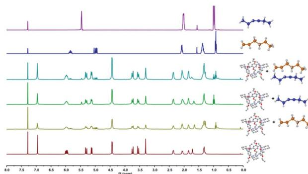
Fig. 2 <sup>1</sup>H NMR spectra (400 MHz, chloroform-d, 298 K) of activated P-TA, activated P-TA after adsorption of vapor 1-He, activated P-TA after adsorption of vapor trans-3-He, activated P-TA after adsorption of the vapor 1-He/trans-3-He mixture for 16 h, 1-He and trans-3-He. The solid samples were dried after vapor adsorption and then dissolved in chloroform-d for analysis.
