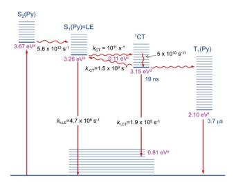
Fig. 7 Diagram of the excited state relaxation processes. <sup>a</sup>From 00-energies of the absorption spectrum; <sup>b</sup>from 00-energies of the emission spectrum; <sup>c</sup>from the Stevens–Ban plot; <sup>d</sup>from b and c; <sup>e</sup>from d– $E_{\text{max}(em)}$ ; <sup>f</sup>see ref. 74.
