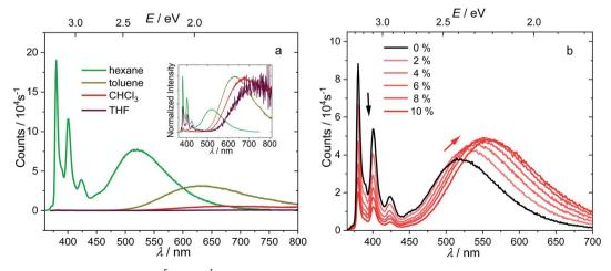
Fig. 4 Emission spectra of 1 ( $c = 1.0 \times 10^{-5}$  mol L<sup>-1</sup>, excitation at 338 nm (3.67 eV)) in solvents with different polarities, with the normalized spectra shown in the inset (a), and in hexane with different percentages of added dioxane with fixed concentration (b).
