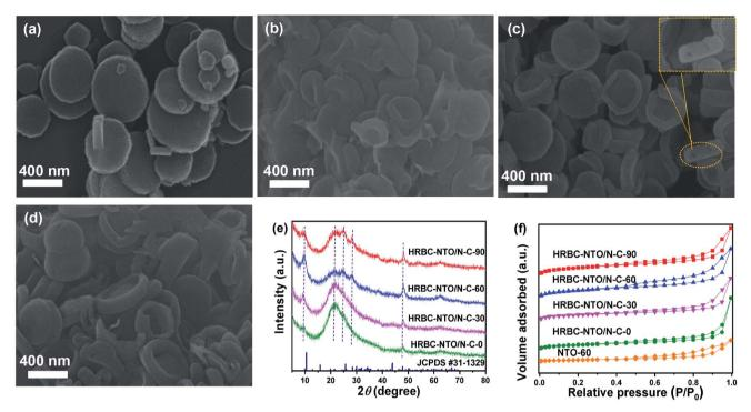
Fig. 3 SEM images of (a) HRBC-NTO/N-C-9, (b) HRBC-NTO/N-C-30, (c) HRBC-NTO/N-C-60, and (d) HRBC-NTO/N-C-90. (e) XRD patterns of HRBC-NTO/N-C-x. (f) N<sub>2</sub> sorption isotherms of HRBC-NTO/N-C-x and NTO-60.
