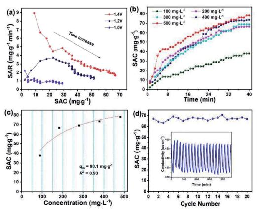
Fig. 7 (a) Ragone plots of SAC vs. SAR of HRBC-NTO/N-C-60 electrodes in different voltage with a flow rate of 25 mL min $^{-1}$ . (b) Desalination curves of HRBC-NTO/N-C-60 in different concentrations of NaCl solution at 1.4 V with a flow rate of 25 mL min $^{-1}$ . (c) Langmuir isotherm of HRBC-NTO/N-C-60. (d) Reusability of the desalination system in a 200 mg L $^{-1}$  NaCl solution at 1.4 V with a flow rate of 25 mL min $^{-1}$ .
