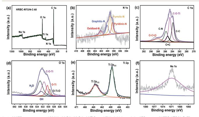
(a) XPS survey spectra and (b) N 1s, (c) C 1s, (d) O 1s, (e) Ti 2p, and (f) Na 1s high-resolution XPS spectra of HRBC-NTO/N-C-60.
