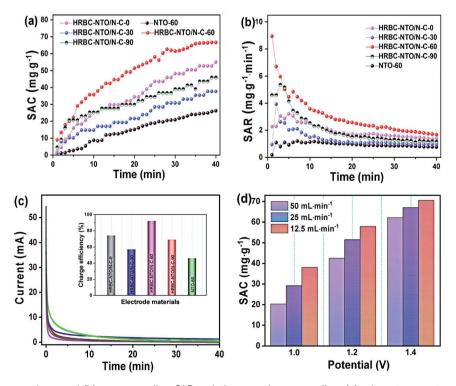
Fig. 6 (a) SAC variations vs. time, and (b) corresponding SAR variations vs. time, as well as (c) relevant current vs. time for all samples in a 200 mg  $L^{-1}$  NaCl solution at 1.4 V with a flow rate of 25 mL min<sup>-1</sup>. (d) The effect of voltage and flow rate on the SAC of HRBC-NTO/N-C-60 in a 200 mg  $L^{-1}$  NaCl solution.
