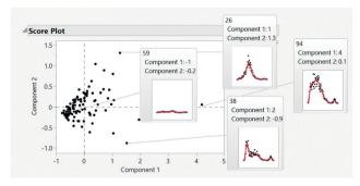
Fig. 20 Functional PCA summarizes the batch information into new coordinate variables that capture variability seen during the batch. In the image, batch curves can be described again using a combination of components 1 and 2.
