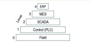
Fig. 6 Simplified hierarchical view of automation infrastructures in the standard ANSI/ISA-95.
