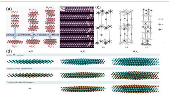
Fig. 1 (a) MAX phases 211, 312 and 413 crystal structures. (b) STEM-HAADF picture of a  $Ti_3C_2T_x$  grain in the (120) zone-axis orientation. (c) Crystal structure of the  $M_3AX_2$  phase with the  $P6_3/mmc$  space group. (d) Mono-transition metal MXene, Solid solution-transition metal MXene, ordereddouble MXene. 20,21,23,24
