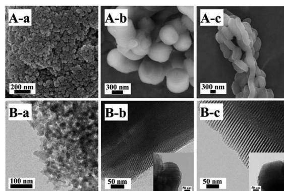
Fig. 5 SEM (A) and TEM (B) images of (a) Z<sub>2</sub>ZnBMMs-100, (b) Z<sub>2</sub>ZnMCM-41-100, and (c) Z<sub>2</sub>ZnSBA-15-100. Inset shows a TEM image of the sample viewed along the hexagonal axis.
