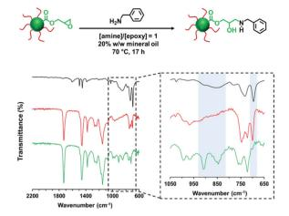
Fig. 4 FT-IR spectra recorded for PLMA<sub>63</sub>-PGlyMA<sub>89</sub> diblock copolymer prior to functionalization (green spectrum), PLMA<sub>63</sub>-PGlyMA<sub>89</sub> diblock copolymer after functionalization with benzylamine (red spectrum) and benzylamine alone (black spectrum). The reaction conditions used are summarized in the corresponding chemical reaction.
