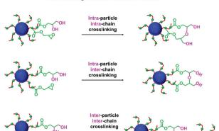
Scheme 3 Schematic representation of the various reactions that can occur when reacting P(LMA $_{50}$ -stat-GlyMA $_{9}$ )-PMMA $_{67}$  nanoparticles with trace water by heating a 20% w/w copolymer dispersion in mineral oil to 110 °C. Following the initial epoxy ring-opening reaction, the resulting hydroxyl groups can react with the remaining epoxy groups. This leads to both intra-particle and/or inter-particle crosslinking.
