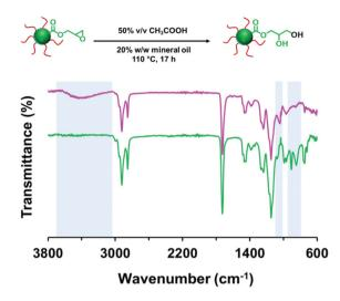
Fig. 7 FT-IR spectra recorded for PLMA $_{63}$ -PGlyMA $_{89}$  prior to (green spectrum) and after reacting with 50% v/v aqueous acetic acid at 110 °C for 17 h (pink spectrum). In principle, this simply involves acid-catalyzed epoxy ring-opening with water but in practice side-reactions also occur, which leads to extensive core-crosslinking of the nanoparticles.
