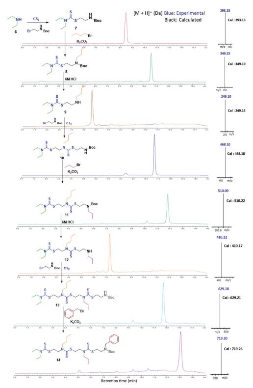
Fig. 1 Assembly of 4-mer SDO1a; left – structure, middle – HPLC, and right – [M + H]<sup>+</sup> in LC-MS. (Boc represents a C(O)O<sup>t</sup>Bu group.)
