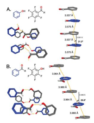
Fig. 1 View of each perspective co-crystal along both the aryl: perfluoroaryl stacks and the hydrogen-bonding pattern. Shorter stacking distances and "tape-like" hydrogen-bonding patterns are observed for ArOH:ArFCHO (A) while longer stacking distances and dimer-like hydrogen-bonding patterns are observed for ArCHO:ArFOH (B).
