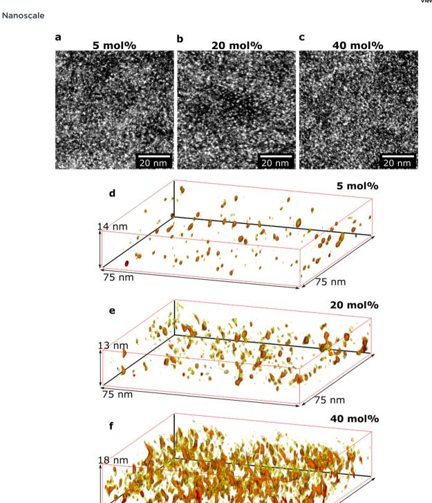
Fig. 2 Electron microscopy (a–c) HAADF-STEM images of representative areas and (d–f) tomography reconstructions of  $p(g_42T-T)$  doped with 5, 20, and 40 mol% Mo(tfd-COCF<sub>3</sub>)<sub>3</sub>, respectively. The sizes of the volumes are marked in nm. Red intensity thresholds in the reconstructions were chosen in order to visualise the position of Mo(tfd-COCF<sub>3</sub>)<sub>3</sub> species. A lower intensity threshold is displayed in yellow.
