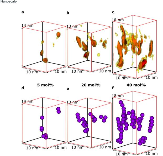
Fig. 3 Representative sub-volumes of the tomographic reconstructions of  $p(g_42T-T)$  doped with 5, 20, and 40 mol% Mo(tfd-COCF<sub>3</sub>)<sub>3</sub>, respectively. (a–c) Reconstructed sub-volumes showing the clusters and (d–f) markers indicate the positions of individual Mo(tfd-COCF<sub>3</sub>)<sub>3</sub> species in the clusters and visualise the gradual change in cluster morphology.
