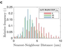
Fig. 4 Histograms from data analysis including all clusters in a volume equivalent to an in-plane area of 150 nm by 150 nm for each sample, displaying distribution of (a) cluster volume, (b) cluster aspect ratio and (c) nearest-neighbour cluster distance. Examples of dopant cluster conformations for different aspect ratios are illustrated as insets in (b).
