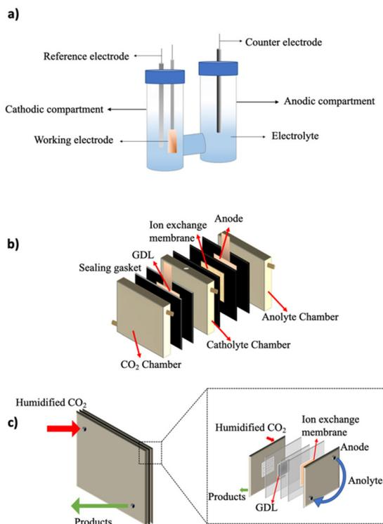
Fig. 2 Illustration of (a) H-cell, (b) flow cell and (c) zero gap MEA electrolyzers used for eCO<sub>2</sub>RR.
