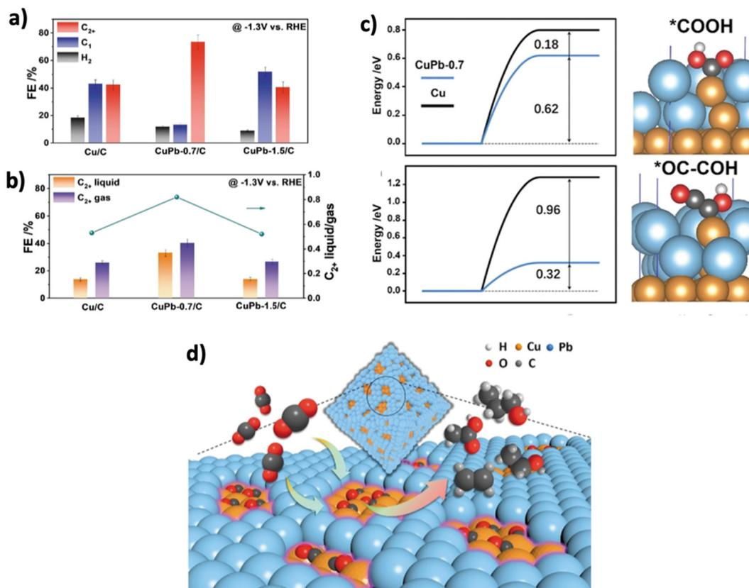
**Fig. 19** (a and b) Faradaic efficiencies of  $C_1$  and  $C_2$  products obtained using a CuPb-0.7/C (where 0.7 represents the thickness of Pb shell) catalyst, (c) simulated data and (d) schematic illustration of the production of  $C_{2+}$  products via the eCO<sub>2</sub>RR route. Reprinted with permission.<sup>265</sup> Copyright 2021, the American Chemical Society.
