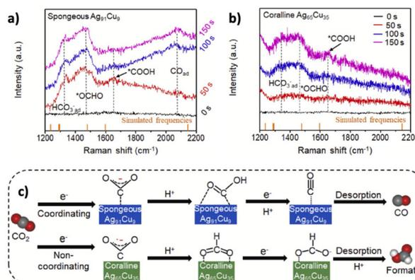
Fig. 7 (a and b) *In situ* Raman spectra obtained during electrolysis and (c) proposed reaction pathways on sponge-like Ag<sub>91</sub>Cu<sub>9</sub> and coralline Ag<sub>65</sub>Cu<sub>35</sub> alloy nanoarchitectures. Reprinted with permission.<sup>73</sup> Copyright 2020, Elsevier Ltd.
