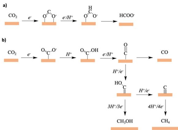
Fig. 3 Illustration of eCO<sub>2</sub>RR pathways for the formation of (a) HCOO<sup>-</sup>, (b) CO, CH<sub>3</sub>OH, CH<sub>4</sub>.
