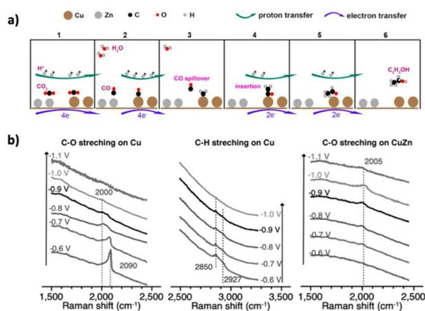
**Fig. 16** (a) Mechanism proposed for ethanol formation using CuZn catalysts. Reprinted with permission.<sup>243</sup> Copyright 2016, the American Chemical Society. (b) Operando Raman spectra obtained during electrolysis of saturated CO<sub>2</sub> in 0.1 M KHCO<sub>3</sub> solution using Cu and CuZn catalysts. Reprinted with permission.<sup>244</sup> Copyright 2019, Wiley-VCH Verlag GmbH & Co. KGaA, Weinheim.
