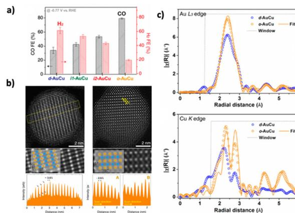
**Fig. 9** (a) Faradaic efficiencies for generation of H<sub>2</sub> and CO using AuCu alloy nanoparticles with designated atomic ordering, (b) high-angle annular dark-field imaging – scanning transmission electron microscope (HAADF – STEM) analysis of ordered AuCu nanoparticles, and (c) XAS analysis of ordered and disordered AuCu nanoparticles. Reprinted with permission.<sup>157</sup> Copyright 2017, the American Chemical Society.
