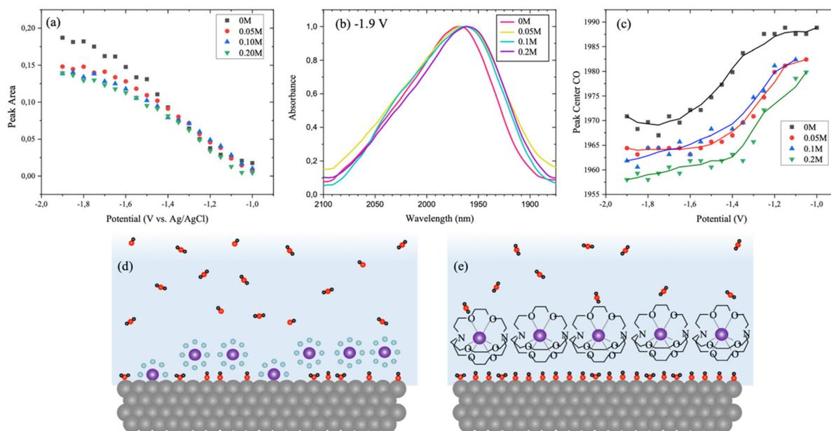
**Fig. 4** Analysis of CO peak (a) CO peak areas changing with potential (b) shift in CO peak at  $-1.9$  V at different cryptand concentrations (c) change in CO peak centers with potential at constant cryptand concentration (d) & (e) schematic representation of cations and cryptates near the catalyst surface.
