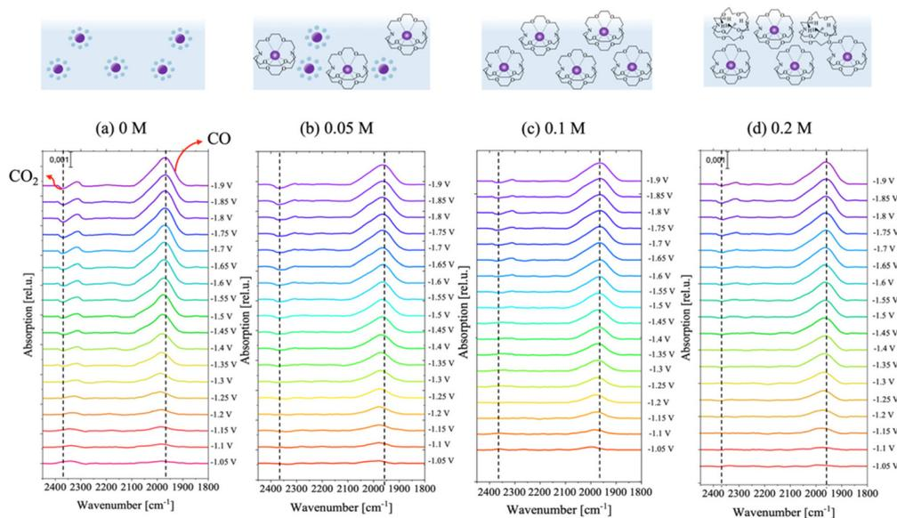
**Fig. 3** *In situ* infrared spectroscopy of the electrode surface with different cryptand concentrations, showing the forward scans obtained through applied potentials  $-1.0\text{ V}$  to  $-1.9\text{ V}$ , revealing the peaks for CO<sub>2</sub> and CO with increasing concentrations (0.2 M to 0.2 M) of cryptands (a–d).
