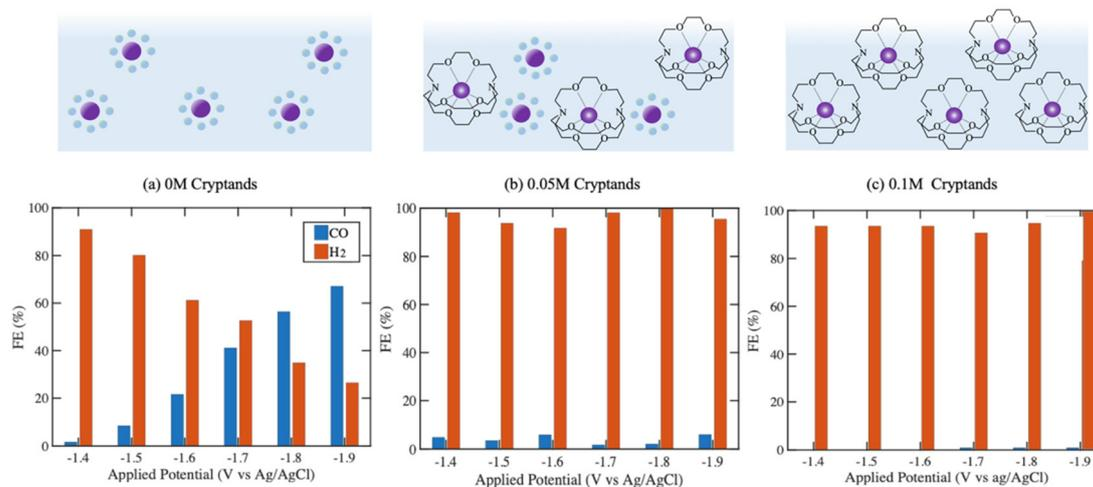
**Fig. 2** Faradaic efficiencies recorded in the H-cell on an Ag catalyst deposited on Ti foil with  $0.1$  M  $KHCO_3$  as the electrolyte, (a) with no cryptands, (b) with  $0.05$  M cryptands, (c) with  $0.1$  M cryptands.
