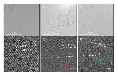
Fig. 3 (a-c) The bright-field TEM image of undoped 2D SnS and 6.4 at% In and 0.1% Bi doped 2D SnS, respectively. (d-e) HRTEM images of the corresponding TEM images in a-c showing the formation of In<sub>2</sub>S<sub>3</sub> and Bi<sub>2</sub>S<sub>3</sub> grains. The sulfide doping formation is in agreement with the oxide counterpart.<sup>22</sup>
