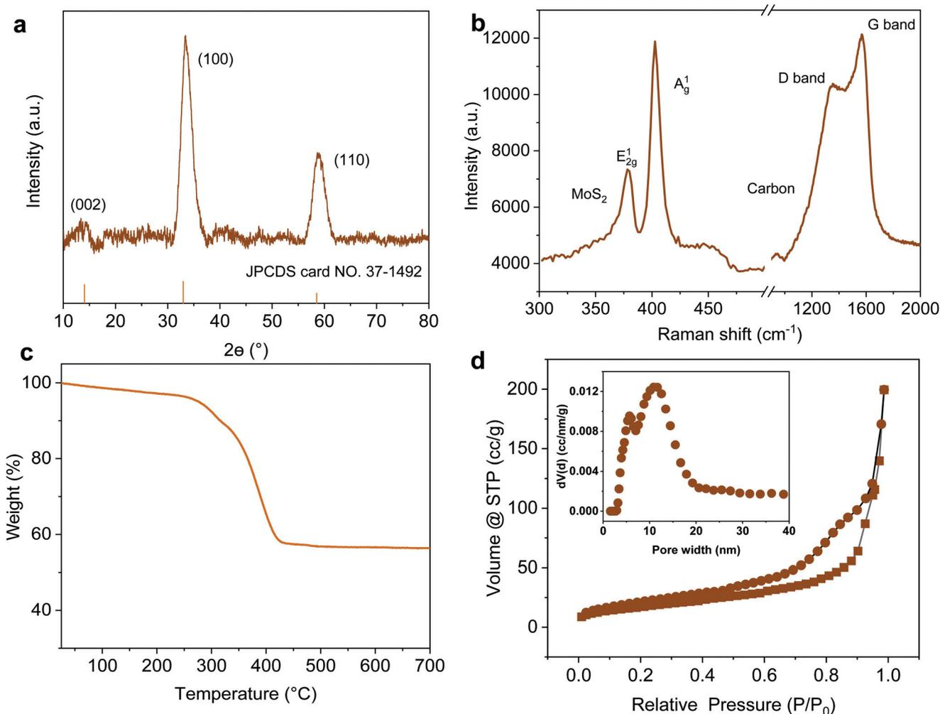
Fig. 3 (a) XRD pattern, (b) Raman spectrum, (c) TGA in air and (d)  $N_2$  adsorption/desorption isotherm curves of  $MoS_2$ -1.5 PNPs; the inset is the curve of pore size distribution.
