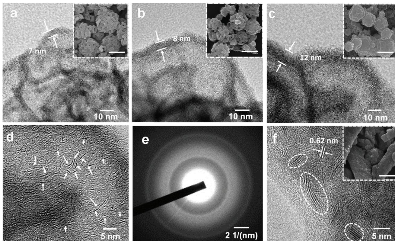
**Fig. 2** TEM images of MoS<sub>2</sub> PNPs prepared at precursor concentrations of (a) 1, (b) 1.5, and (c) 3 mg mL<sup>-1</sup>. The insets are the corresponding SEM images with a scale bar of 500 nm. (d) HRTEM image and (e) SAED pattern of MoS<sub>2</sub>-1.5 PNPs. (f) HRTEM image of bulk MoS<sub>2</sub> prepared without any polymer template; the inset is the corresponding SEM image with a scale bar of 500 nm.
