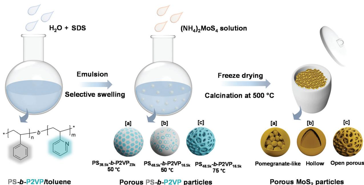
**Scheme 1** Synthesis strategy of MoS<sub>2</sub> particles with various morphologies using PS-*b*-P2VP as a sacrificial soft template.
