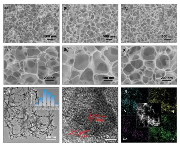
Fig. 2 ( $a_1-a_2$ ) SEM images of N-doped graphitic carbon. ( $b_1-b_2$ ) SEM images of VN/NC. ( $c_1-c_2$ ) SEM images of Co-VN/NC. (d) TEM images of 3D Co-VN/NC, inset: size distribution of the Co-VN nanocrystals in 3D Co-VN/NC. (e) HRTEM images of Co-VN/NC. (f) EDS mappings of Co-VN/NC.
