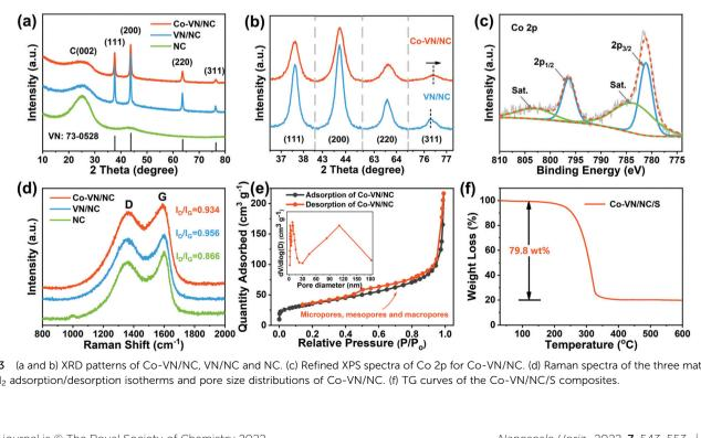
Fig. 3 (a and b) XRD patterns of Co-VN/NC, VN/NC and NC. (c) Refined XPS spectra of Co 2p for Co-VN/NC. (d) Raman spectra of the three materials. (e) N2 adsorption/desorption isotherms and pore size distributions of Co-VN/NC. (f) TG curves of the Co-VN/NC/S composites.
