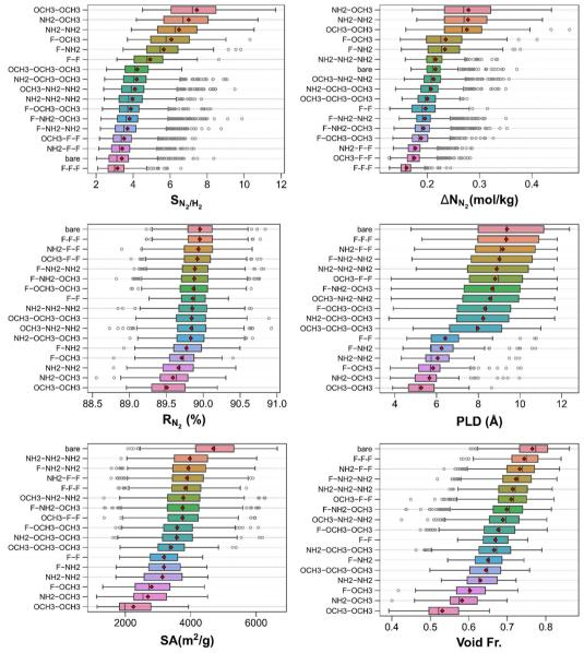
Fig. 6 Classification of N<sub>2</sub>/H<sub>2</sub> separation performance metrics and structural features of MOFs by functional groups
