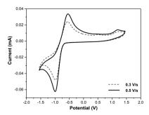
Fig. 2 Solid-state cyclic voltammetry of Per-MOF in CH<sub>3</sub>CN using TBAPF<sub>6</sub> 0.1 M as electrolyte at different scan rates. Platinum wire was used as the counter electrode and silver wire as the pseudoreference electrode. Ferrocene was added as internal standard. All potentials are reported versus Ag/AgCl.
