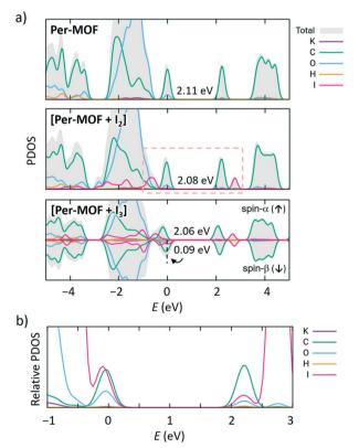
Fig. 5 a) Atom-projected density of states (PDOS) and bandgap values calculated for Per-MOF, [Per-MOF +  $I_2$ ] and [Per-MOF +  $I_3$ ] at the HSE06 level. Spin- $\alpha$  and spin- $\beta$  channels (with their corresponding bandgaps) are indicated in [Per-MOF  $+ I_3$ ]. The Fermi level was set to the valence band maximum. b) Relative PDOS of [Per-MOF + I2] calculated as the PDOS divided by the number of atoms of each type in the unit cell.
