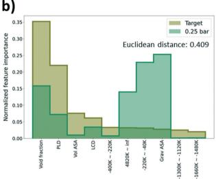
Fig. 6 Feature importance values for the top 10 important features at the target domain. Normalized feature importance values of the target domain and a) the best source domain, gas uptake at 100 bar. b) The worst source domain, gas uptake at 0.25 bar. The best source domain is colored navy and the worst source domain is colored green.
