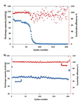
Fig. 7 Long term cycling (blue) and coulombic efficiency (red) of (a) NMO and (b) NMCO for 200 cycles at C/2 (after a pre-conditioning for 5 cycles at C/10).
