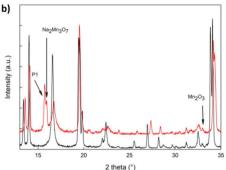
Fig. 3 The XRD patterns in the whole angular range (a) and in a limited zone (b) of NMO and NMCO samples. The main peaks of the secondary phases are indicated
