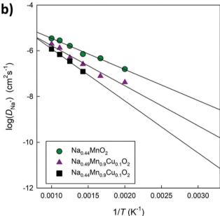
Fig. 12 Arrhenius plot of Na<sup>+</sup> diffusion coefficients (D) for (a) two different models having the same composition (Na<sub>0.44</sub>MnO<sub>2</sub>) and characterized by a different distribution of Na+ ions between 1D and 2D channels; and (b) three different models having the same occupation of the Na1 site (60%) but different composition.
