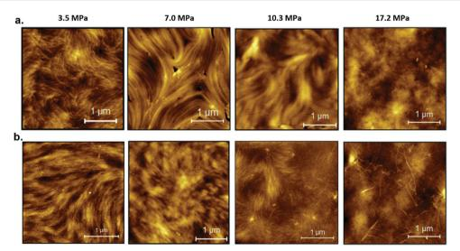
Fig. 2 Atomic force microscopy images of PBTTT-C<sub>14</sub> films formed in supercritical (a) pure n-pentane and (b) n-pentane: toluene at different pressures.
