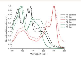
Fig. 1 Normalized UV-vis absorption spectra of polymers P1-P3 in a solution of CHCl<sub>3</sub> and as a thin film.
