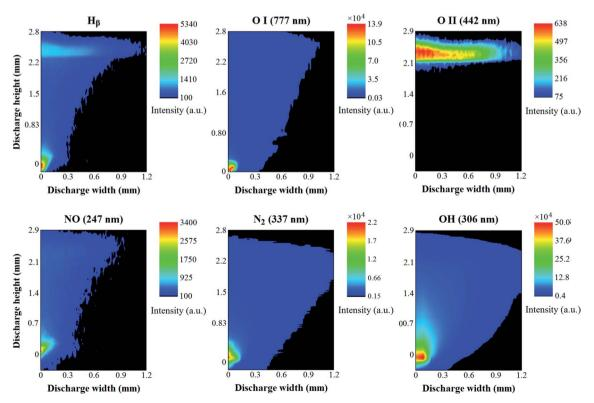
Fig. 5 2-D emission profiles of the background species (H, O I, O II, NO, N<sub>2</sub> and OH) in HDC-APGD
