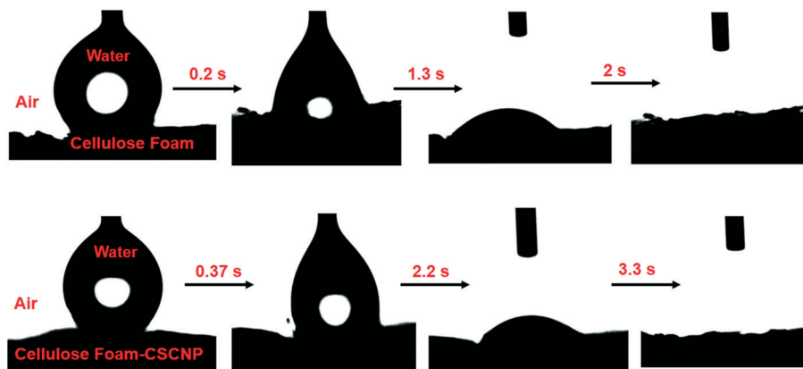
Fig. 5 Water contact angle measurements reveal the hydrophilic nature of the CF and CF-CSCNP surfaces, and indicate the water soaking behaviors with respect to time, captured through different image frames using a contact angle meter.
