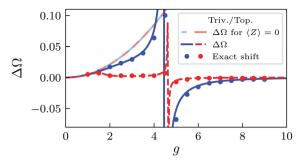
Fig. 4 Plot of  $\Delta\Omega$  (egn (18)) vs. q for both the trivial (blue) and topological (red) phase. The comparison with  $\Delta\Omega$  calculated with  $\langle Z \rangle$  has been included in lighter colors. The dots corresponds to the exact shift (eqn (10)). Parameters:  $\Omega$  = 10,  $\delta$  =  $\pm$ 0.6, N = 20,  $n_{\text{max}}$  = 60.
