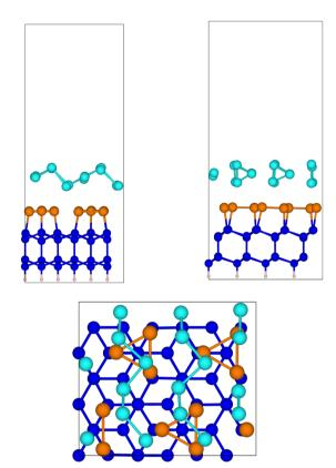
Fig. 7 Side and top views of the relaxed configuration of tellurene in the Te(1010) geometry on Si(111)- $(\sqrt{3} \times \sqrt{3})R30^{\circ}$ -Sb surface.
