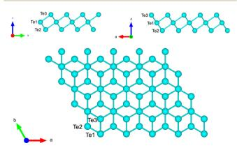
Fig. 2 Side and top views of the optimized structure of tellurene in the 1T-MoS<sub>2</sub>-like geometry. The three atoms per unit cell are labelled
