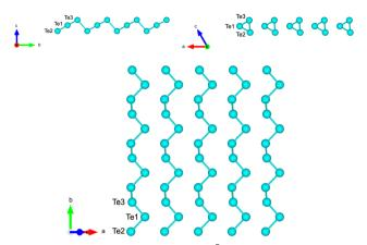
Fig. 3 Side and top views of the Te(1010) trilayer slab in the initial geometry obtained by truncation of the bulk. The three atoms per unit cell are labelled.
