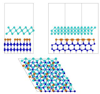
Fig. 5 The relaxed configuration of tellurene in a trilayer 1T-MoS<sub>2</sub>-like geometry adsorbed on the Si(111)- $(\sqrt{3} \times \sqrt{3})R30^{\circ}$ -Sb surface in a slab geometry. Side and top views are shown
