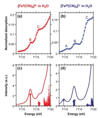
Fig. 2 Experimental (top) and simulated (bottom) Fe K-edge XANES spectra of  $[Fe^{II}(CN)_6]^{4-}$  and  $[Fe^{III}(CN)_6]^{3-}$  simulated results have been blue-shifted by 143.0 eV to match the experiment. The A and B features in the two complexes are quadrupolar transitions from the Fe 1s  $\rightarrow$  3d orbitals. Reproduced with permission from ref. 84. Copyright 2018 American Chemical Society
