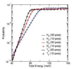
Fig. 7 Transmission probabilities through GDY of  $H_2$  (blue),  $D_2$  (red) and  $T_2$  (black) for perpendicular incidence within the 3D-TDWP calculations (full lines) and the 1D model (open circles) as functions of total energy (meV).
