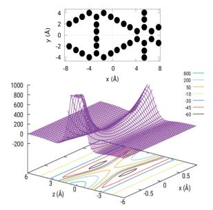
Fig. 2 Upper panel: GDY unit cell employed in the 3D-TDWP calculations, with indication of the coordinate system used. Lower panel: H2-GDY interaction potential (vertical axis, in meV) as a function of x and z (in Å), around the center of the pore, with y = 0.
