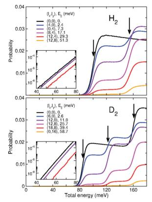
Fig. 3 3D-TDWP transmission probabilities for H<sub>2</sub>-GDY (upper panel) and D<sub>2</sub>-GDY (lower panel) as functions of the total translational energy (meV) for different incidences  $(l_x, l_y)$ . The corresponding parallel energies  $E_{\parallel}$   $(l_x, l_y)$ (eqn (7)) are indicated in the legends. Arrows show the energy levels of the transition state (Table 2). Insets depict the behavior of some of the probabilities in the low energy range. See text for discussion.
