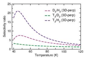
Fig. 8 Selectivity ratios for D<sub>2</sub>/H<sub>2</sub>, T<sub>2</sub>/D<sub>2</sub>, and T<sub>2</sub>/H<sub>2</sub> as functions of temperature (K), as estimated from the 1D model.
