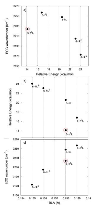
Fig. 7 Correlation between physical quantities sensitive to  $\pi$ -electrons conjugation. Panel a: ECC phonon wavenumber vs.  $\Delta E$  ( $\Delta E$  is the relative crystal energy – per atom – referred to graphene, see text). Panel b:  $\Delta E$  vs. BLA parameter. Panel c: ECC phonon wavenumber vs. BLA. The data corresponding to 6-h<sup>3</sup>L crystal are highlighted by a red circle.
