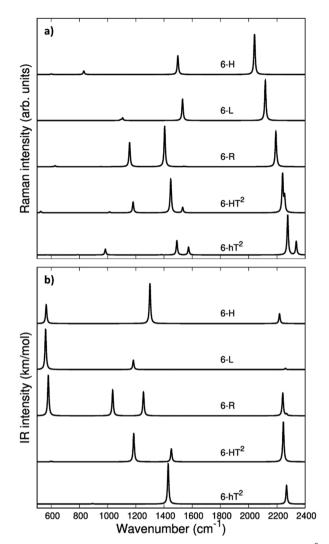
Fig. 3 Computed Raman (a) and IR (b) spectra of GDY systems: 6-hT<sup>2</sup>, 6-HT2, 6-R, 6-L and 6-H
