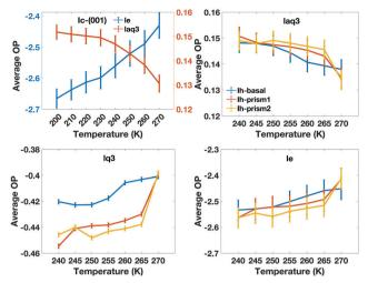
Fig. 9 The average value of  $laq_3$ ,  $lq_3$ , and le for the liquid-like molecules on the Ih surfaces and the average value of  $laq_3$  and le for the liquid-like molecules on the Ic-(001) surface as a function of temperature.
