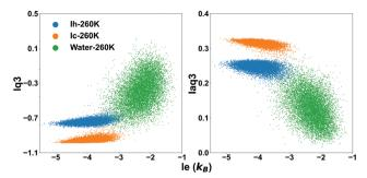
Fig. 3 The distribution of the values of the local entropy fingerprint le and either or lag<sub>3</sub> for bulk water (green dots), Ih (blue dots) and Ic (orange dots) at 260 K
