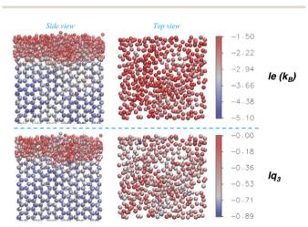
Fig. 10 The spatial distribution of the order parameters le (top panels) and  $lq_3$  (bottom panels) in exemplary MD snapshot of a Ih prism2 surface at 270 K, viewed from the side (left) and top (right) with respect to the surface. Only oxygen atoms are shown, coloured according to the value of the order parameters. The thresholds of for the crystal/liquid classification are  $-3.17~k_{\rm B}$  for le and and -0.67 for  $lq_3$ .
