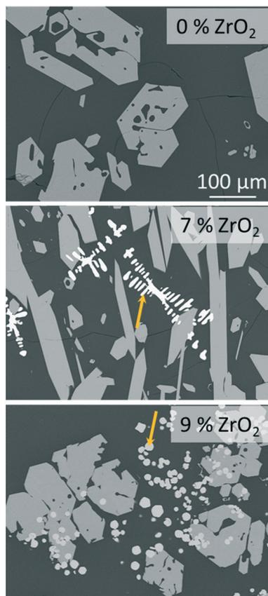
Fig. 2 SEM micrographs (backscattered electrons) of samples Zr0, Zr7, and Zr9 after slow cooling to room temperature at identical magnifications. The arrows point at ZrO<sub>2</sub> precipitates.
