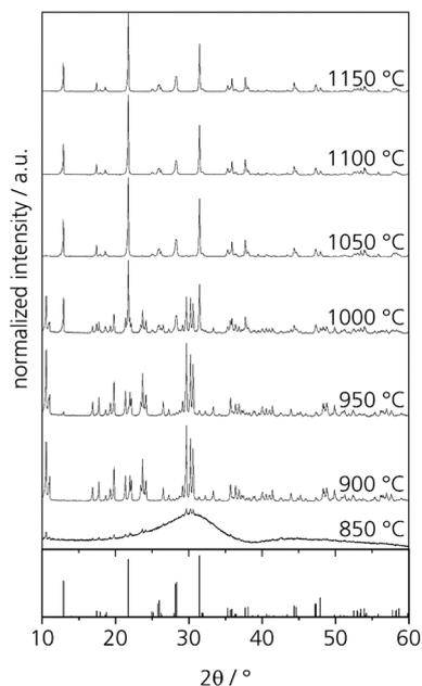
Fig. 5 XRD patterns of glass Zr0 after heat treatments for 5 h at different temperatures. The theoretical peaks displayed at the bottom are attributed to  $\text{NaYSi}_2\text{O}_6$  (calculated from ICSD 171255, ref. 16).
