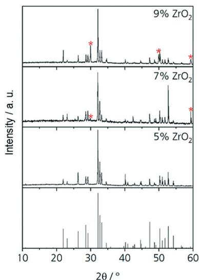
Fig. 3 XRD patterns of Zr5, Zr7, Zr9 and Zr11 after slow cooling to room temperature. The theoretic pattern at the bottom belongs to  $NaY_9Si_6O_{26}$  (JCPDS no. 00-035-0404). The peaks of cubic zirconia (JCPDS no. 01-077-2112) are marked with red stars.
