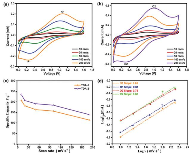
Fig. 4 Cyclic voltammetry curve of (a) **TDA-1**. (b) **TDA-2**. (c) The specific capacitance of **TDA-1** and **TDA-2** electrodes at different scan rates. (d)  $b$ -value in eqn (1) at two pairs redox peaks.
