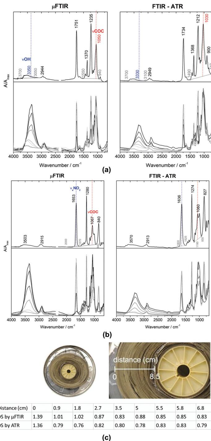
**Fig. 9** Micro FITR ( $\mu$ -FTIR) in transmission mode and ATR-FTIR spectra of (a) CA and (b) CN, where 3330, 1030  $\text{cm}^{-1}$  and 1636, 1060  $\text{cm}^{-1}$  are used to produce DS values. (c) DS values of CA of a historical reef from the inner parts to outer parts acquired using  $\mu$ -FTIR and ATR-FTIR. Reproduced with permission,<sup>155</sup> copyright (2020) Springer Nature.
