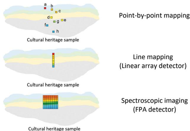
**Fig. 2** Schematic of point-by-point mapping, line mapping and spectroscopic imaging. The colours of pixels represent concentration of an investigated component. Red/orange colours represent a high concentration of the component while blue/green region shows a low concentration.
