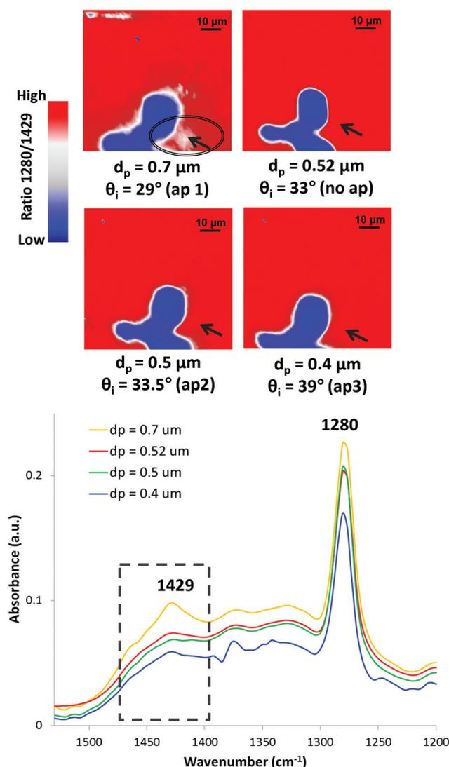
Fig. 10 Depth profiling of the surface of the CN jewellery box using micro ATR-FTIR spectroscopic imaging in the area corresponding to blistering. Reprinted with permission.<sup>187</sup>
