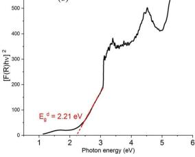
Fig. 6 Optical absorption spectrum (a) and Tauc plot of  $[F(R)*h\nu]^2$  vs.  $h\nu$  (b).
