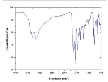
Fig. 4 The infrared absorption spectra of (C<sub>5</sub>H<sub>8</sub>N<sub>3</sub>)[CuCl<sub>3</sub>], dispersed in a KBr pellet
