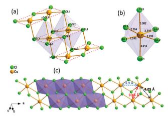
Fig. 2 Detailed presentation of the inorganic polymeric fragment: (a) description of the Cl and Cu ion environments, (b) geometric description of the CuCl<sub>6</sub> octahedron, and (c) view of a single  $[CuCl_3]_{\infty}$  inorganic chain.
