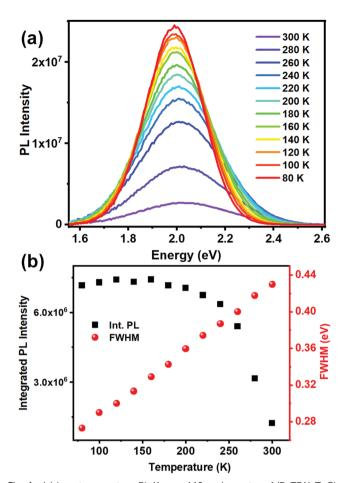
Fig. 4 (a) Low temperature PL ( $\lambda_{\rm exc}$  = 440 nm) spectra of (BzTEA)<sub>2</sub>TeCl<sub>6</sub> crystals; (b) integrated PL intensity and bandwidth (FWHM) as a function of temperature.
