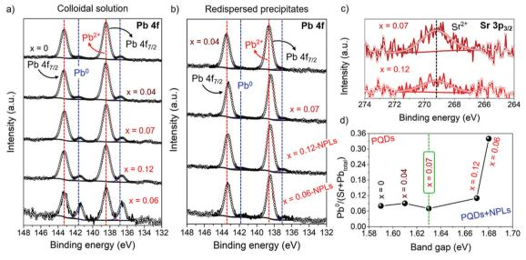
Fig. 3 High-resolution (HR) XPS spectra of (a and b) Pb 4f, (c) XPS Sr 3p<sub>3/2</sub> and (d) calculated metallic Pb-to-(Sr + Pb<sub>total</sub>) ratio for (a, c and d) FAPb<sub>1-x</sub>Sr<sub>x</sub>I<sub>3</sub> PQDs colloidal solutions, and (b) their corresponding redispersed precipitates.
