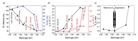
Fig. 5 (a) Behavior of the PL lifetime and PLQY, (b) radiative  $(k_r)$  and non-radiative recombination  $(k_{nr})$  decay rate constants, and (c) their corresponding  $k_{nr}/k_r$  ratio for the FAPb<sub>1-x</sub>Sr<sub>x</sub>l<sub>3</sub> PQDs colloidal solutions by varying the Sr fraction.
