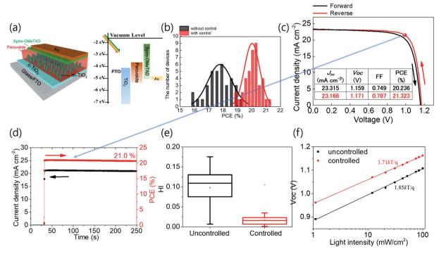
Fig. 6 (a) Structure and energy diagram of OIHPs; (b) distribution of PCEs for controlled and uncontrolled OIHPs; (c and d) j-V curve for a champion cell with optimisation and current-density values at a steady  $V_{\text{max}}$ ; (e) HI and (f) ideality factor for the cell with and without optimisation.
