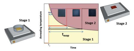
Scheme 1 Fabrication process for perovskite films and XRD data for the wet film and completed perovskite for MAPbI<sub>3</sub>.
