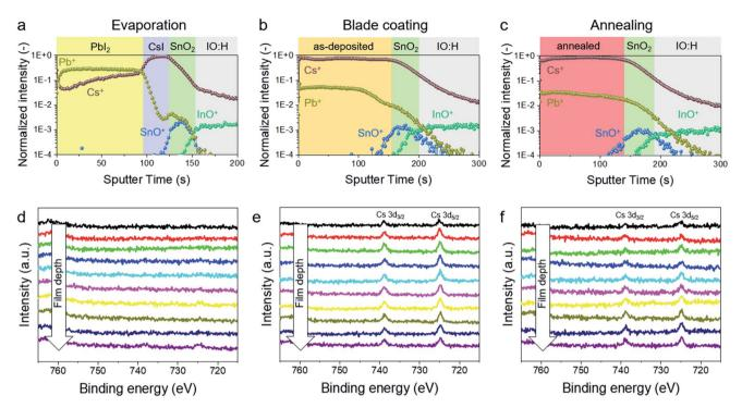
Fig. 3 ToF-SIMS depth profile of (a)-(c) cation species at different stages of the hybrid PVD/blade coating process and XPS with depth profiling (d)-(f) of the stack after each step of the coating process. XPS Cs 3d spectra after (a) evaporation, (b) blade coating and (c) annealing. The ten lines correspond to profiles at 0 nm, 10 nm, 20 nm, 30 nm, 40 nm, 80 nm, 120 nm, 160 nm, 200 nm and 300 nm depth.
